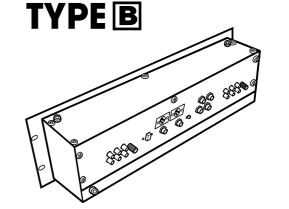
Initially, the I/O panel is placed on the top-side. In case of changing the jack panel position to TYPE B, please use following instructions.
